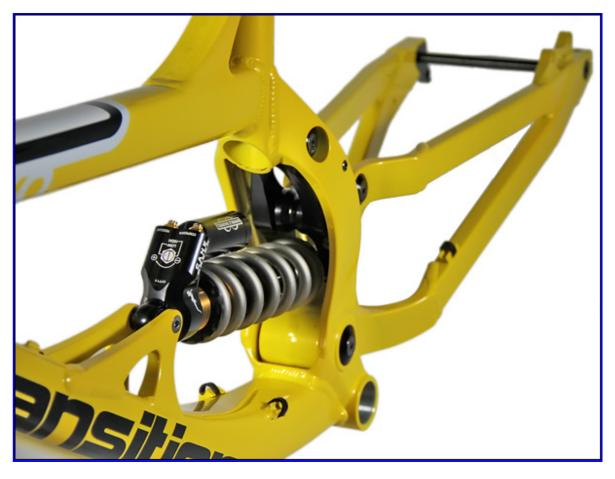
The cable routing on the TR450 worked quite well. The rear derailleur cable runs through the rear chainstay. On some internal cable routing designs it can be hard to snake the cable through the chainstay but the TR450 was pretty easy, as the cable is partially accessible from the inside of the backside of the chainstay.
